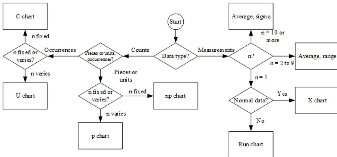
Figure 1: Control chart selection flow diagram
