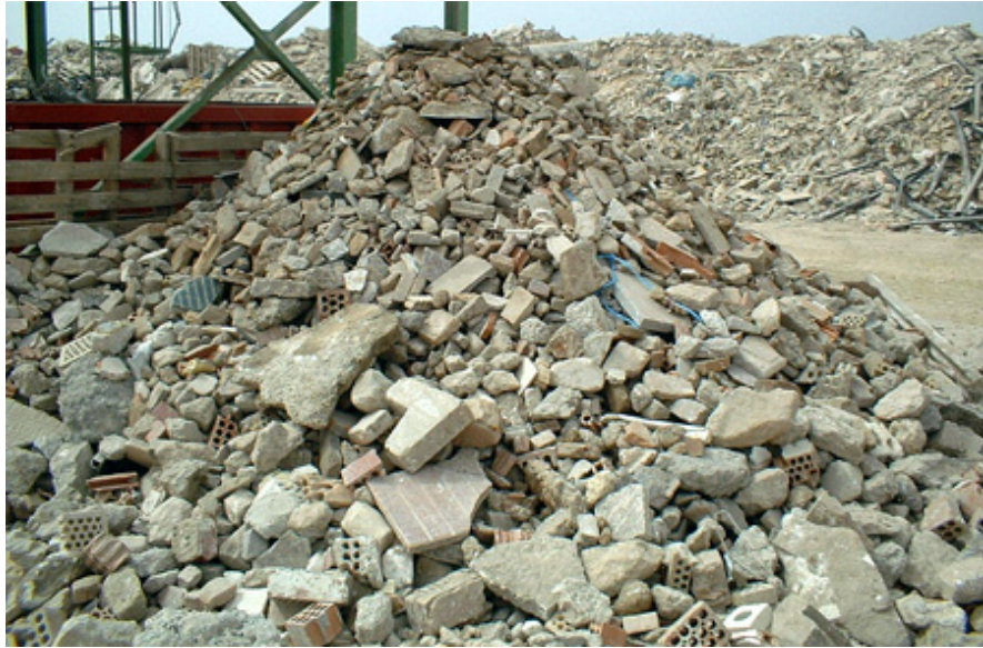
Figura 5.10 Material Mayor a 40 mm. Fuente: Recovery S.A. 2006
